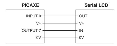
Note: The connections must be made directly to the PICAXE output pins (not via the darlington driver buffered outputs found on the PICAXE starter pack project boards)
