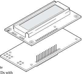
Note that the LCD is fitted above the TRACK side of the PCB. Ensure no solder bridges between pins on the header.
