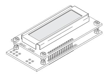
The serial LCD and clock module allows microcontroller systems (e.g. PICAXE) to visually output user instructions or readings, without the need for a computer. This is especially useful when working, for example, with analogue sensors, as the analogue reading can easily be displayed on the LCD module. All LCD commands are transmitted serially via a single microcontroller pin using the **serout** command. e.g.
